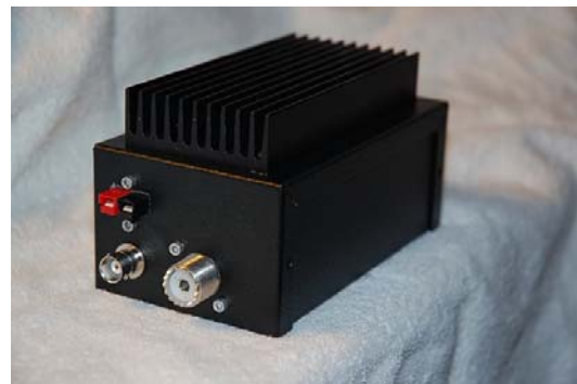
DC Input; RF In; RF Out
